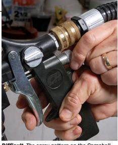
**Difficult.** The spray pattern on the Campbell Hausfeld guns is adjusted by changing the fluid and airflow knobs in tandem with the air cap. The system made it tough to get a nice pattern.
