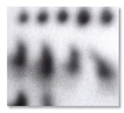
**Poor pattern.** A sloppy or pear-shaped spray pattern makes it almost impossible to blend overlapping strokes together.
