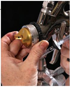
**Innovative and easy.** The gun from the Apollo 835 Turbospray has a dedicated ring near the front that makes it easy to adjust the width of the spray pattern.
