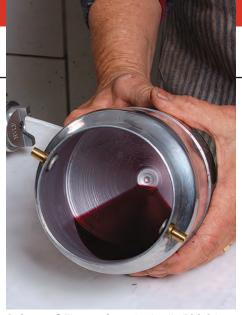
**Spit proof.** The cup from the Apollo ECO-3/ E7000 system has a cone-shaped bottom, which helps keep the gun from picking up air when the fluid gets low—a helpful feature.
