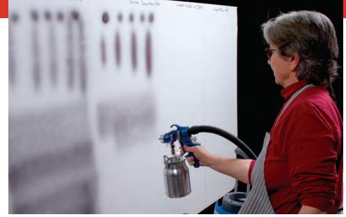
**Best test.** Masaschi tested each system by spraying dark-colored solvent-based and water-based lacquer onto white cardboard, making it easy to see the size of the spray droplets and the shape of the spray pattern.
