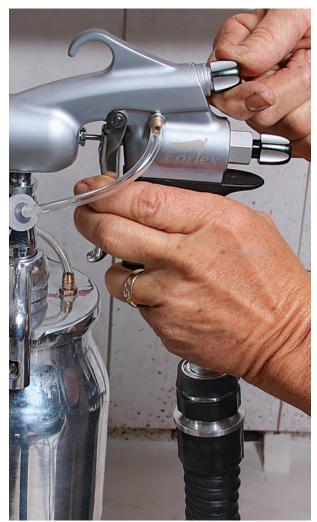
**Conventional controls.** Many guns have separate knobs that adjust the fluid volume and the air volume, which in turn control the width of the spray pattern. This traditional system, as seen on the Earlex SprayPort, is straightforward.
