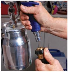
**Out of the way.** The hose on the Fuji Spray Mini-Mite 3 attaches out of the way at the end of the handle, and has an easy-to-grip coupling that makes it a snap to attach.
