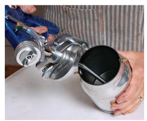
**Coating protects.** The Earlex SprayStation and the Apollo 835 Turbospray both have cups with a protective coating inside that guards against corrosion.
