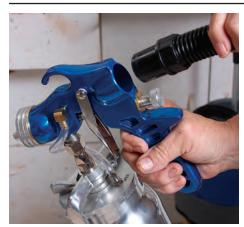
**In the way.** The hose on the Earlex SprayStation is close to the fluid-adjustment knob underneath, making it harder to turn the knob, and also to spray in tight spaces.
