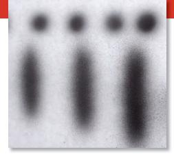
**Good pattern.** You want a tapered, symmetrical spray pattern that makes it easy to lay down an even coat of finish and overlap strokes without leaving lines behind.
